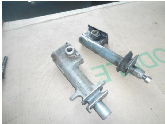
Cast Housing Replaced by a Welded one
